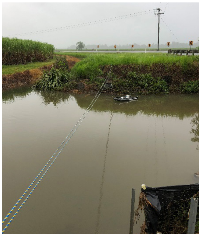
Figure 7: Moving Boat Measurement
